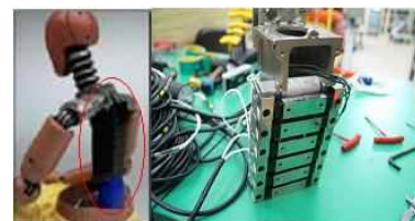
Fig.3 Spine Box Assembly with Rib Load cells
