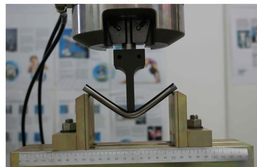
Fig. 3 Three-point Bending Test
