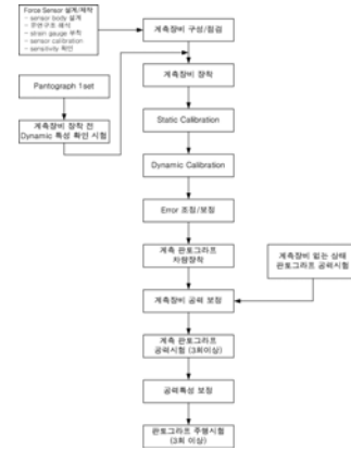
Fig. 4 Typical Flow Chart of Test Procedure
