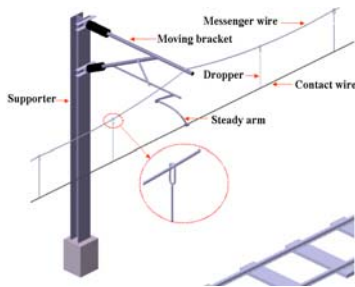
Fig. 2 Schematic view of catenary system in high-speed line
