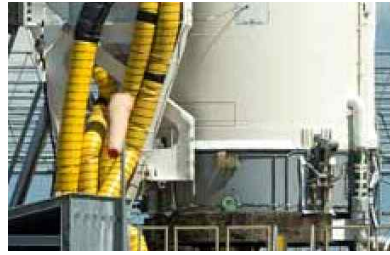
Fig. 2 Antares 1st stage fuel umbilical connection
