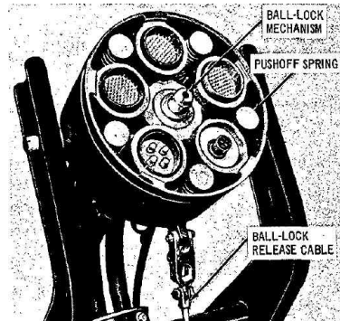
Fig. 3 Jupiter 1st stage electrical umbilical connection [1]
