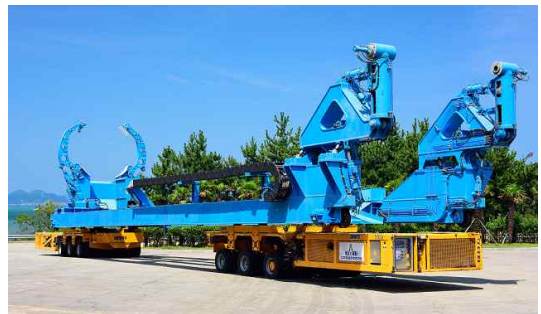
Fig. 6 SPMT and transporter erector for KSLV-I.
