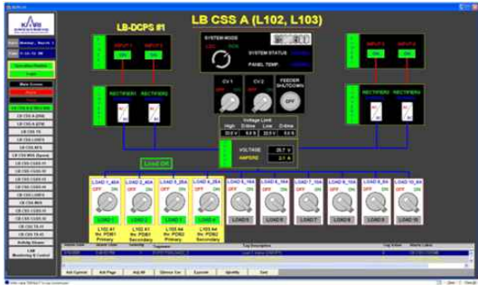
Fig. 5 EWS Operational Interface of DCPS
