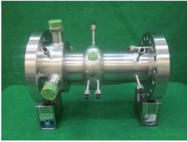
Fig. 6 One-body Pre-burner [17]
