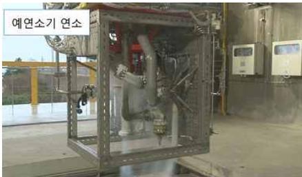
Fig. 19 Power-pack Combustion Test.
