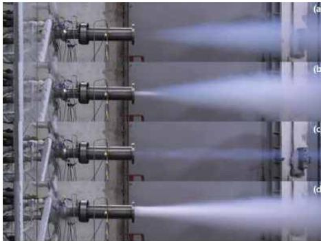
Fig. 7 Combustion Test of Pre-burner [17]
