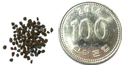
Fig. 3 Fabricated MnO 2 /γ-Al 2 O 3 catalyst
