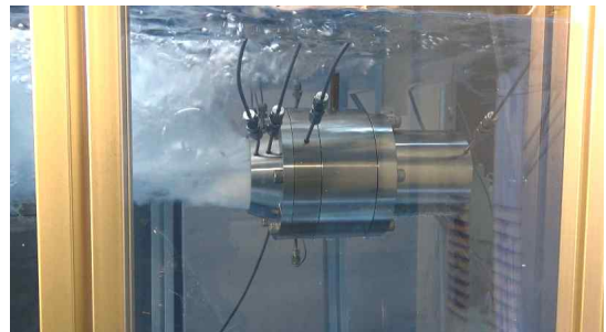
Fig. 8 Underwater jet propulsion system operation test
