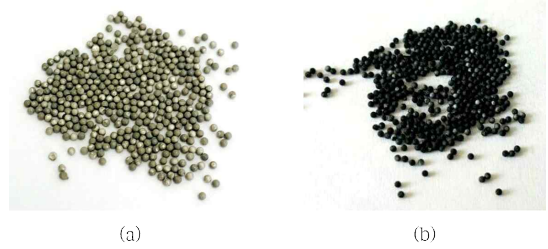
Fig. 1 (a)Pt/Al 2 O 3 bead (b)Cu/Al 2 O 3 bead.
