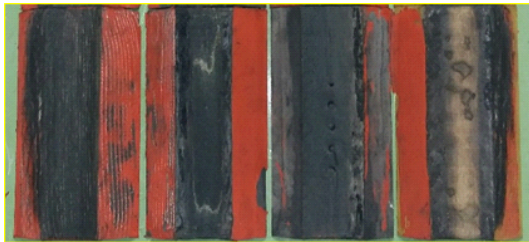
Fig. 6 Surface shape of test samples after test. (Sample 4, 3, 2, 1 from left, respectively)
