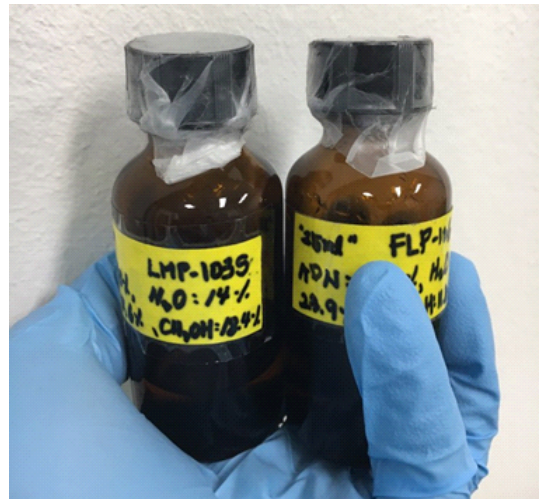
Fig. 2 Fabricated ADN-based monopropellants
