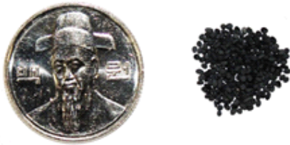
Fig. 3 Fabricated Pt-Cu/LHA catalyst
