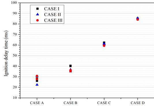
Fig. 5 Ignition delay time by ignition position and time
