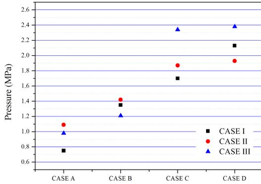
Fig. 3 Combustion chamber pressure peak value
