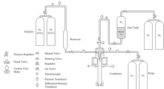
Fig. 1 Schematic of propellants supply lines
