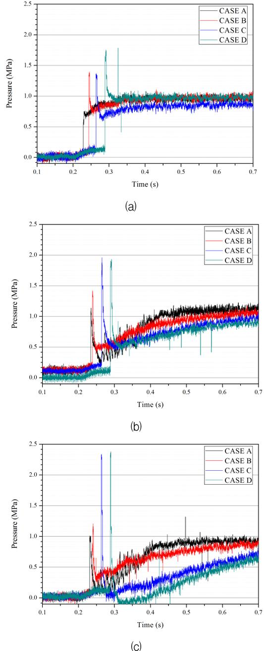
Fig. 2 Combustion chamber pressure under different conditions: a) CASE I; b) CASE II; c) CASE III
