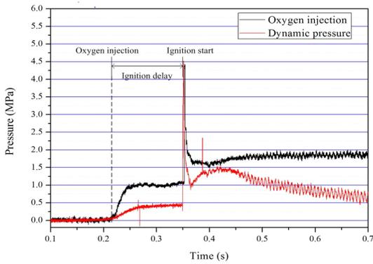
Fig. 4 Calculation method of ignition delay time
