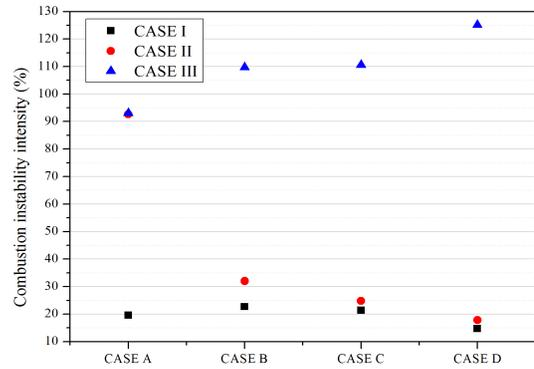
Fig. 6 Combustion instability intensity by ignition position and time
