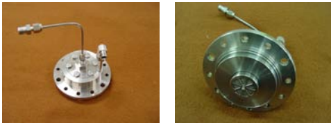
Fig. 3 H 2 O 2 used catalyst bed
