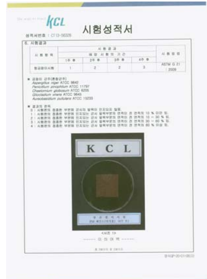
Fig. 2. Test result of fungi incubation of P50
