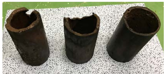
Fig. 11 Fuel grain after the test
