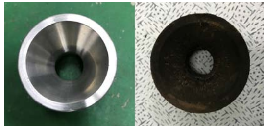
Fig. 13 Nozzle before and after test
