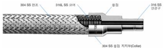
Fig. 6 Stainless steel flexible hose (sample)
