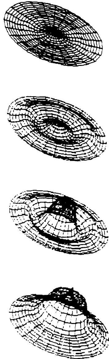
Fig. 20. 3-D plots of circular sawblade at normal direction of measurement due to change of rotating speed.
