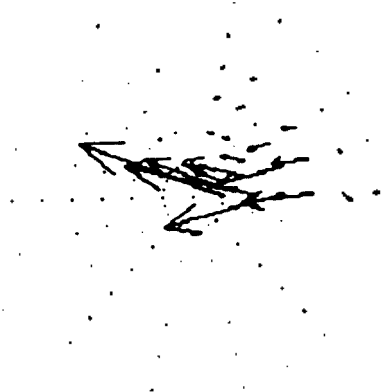
Fig. 22. Acoustic intensity vector flow due to rotating speed for tangential-radial plane.
