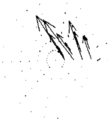
Fig. 23. Acoustic intensity vector flow due to rotating speed for radial-normal plane.
