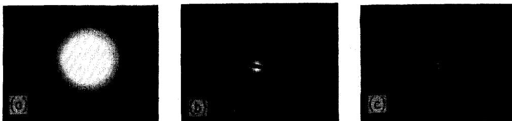
Fig. 5. TEM diffraction patterns of PI films (a) deposited with neutral cluster beam, (b) deposited with ICB at I_c=15 mA, V_c=200 V, and V_a=400 V, (c) deposited with ICB at I_c=15 mA, V_c=200 V, and V_a=800 V.
