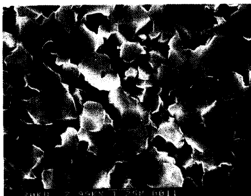
그림 1. Surface morphology of CdS films grown on the pyrex plate by HWE. Source temp. 610°C ; Substrate temp. 480°C .
