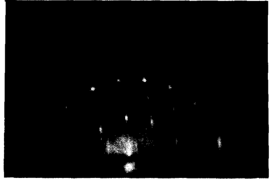
Fig. 3. RHEED pattern obtained from 1-D (3×1) structure formed by Mg-depositing on the Si(111)7×7 surface at 450°C.
