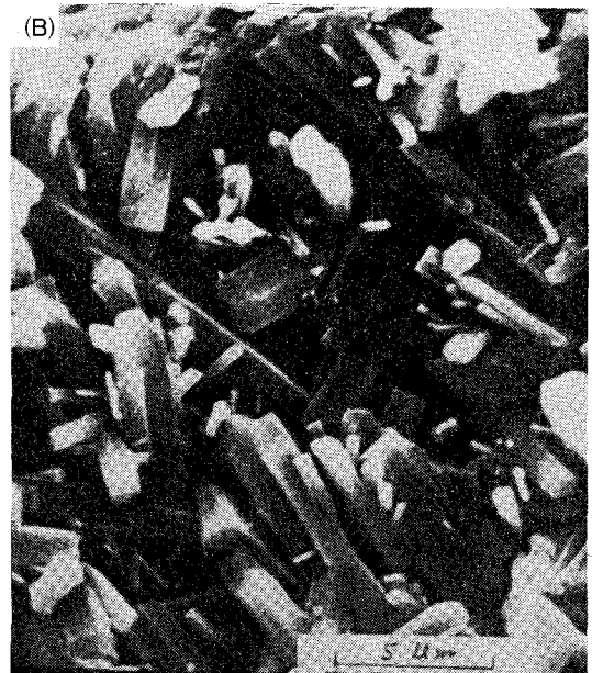
〈그림-2〉 Scanning electron micrographs of clinker containing large amount of \beta - C_2S and C_1A_1\bar{S} (A) and 1 day hydrated cement showing of ettringite.
