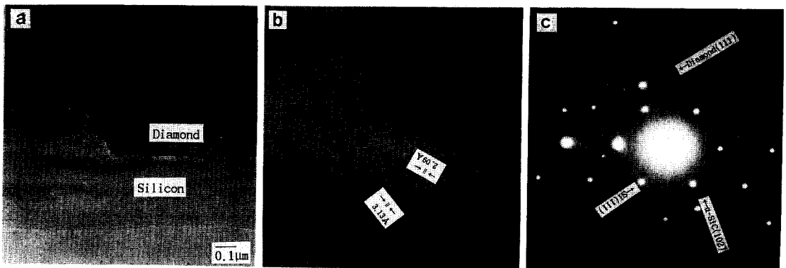
Fig. 4. (a) Cross-sectional TEM micrograph of the film at 60 torr, (b) Corresponding high resolution TEM micrograph, (c) Corresponding SAED pattern.
