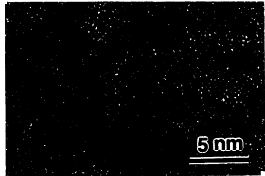
Fig. 4. HRTEM micrograph showing the crystallites in the amorphous matrix.
