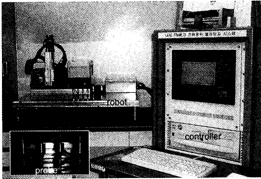
Fig. 5. Photograph of the residual stress measurement system constructed in this work.
