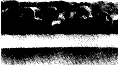
Fig. 6. TEM photograph of the sol-gel derived \text{La}_{2/3}\text{Sr}_{1/3}\text{MnO}_3 thin film on \text{SiO}_2/\text{Si}(100) substrate.
