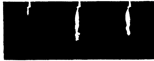
0.1MPa 0.4MPa 0.7MPa Fig. 8 Spray of LPG at 50ms after injection-500K
