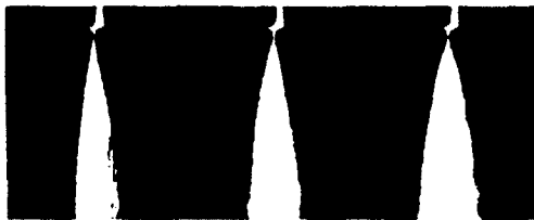
0.1MPa 0.4MPa 0.7MPa Fig. 6 Spray of Diesel at 50ms after injection-298K
