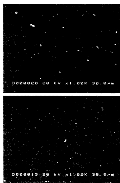
Fig. 3. SEM images showing surface microstructures of (a) Y_2O_3 /Ni-W and (b) YBCO/ Y_2O_3 /Ni-W.
