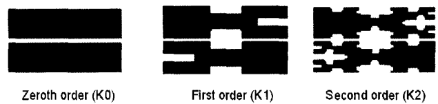
Fig. 2. Two port Koch fractal shape coupler.
