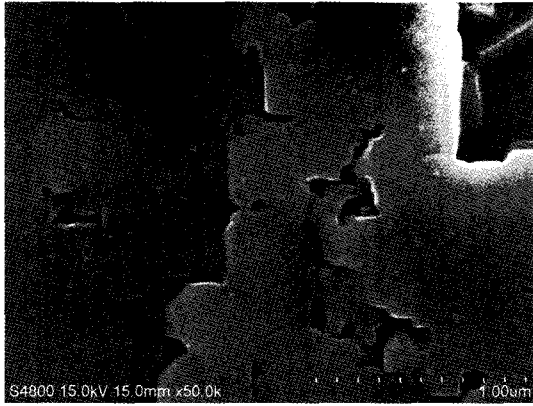
Fig. 7. SEM image of the \text{Sm}_{1+x}\text{Ba}_{2-x}\text{Cu}_y\text{O}_{7-\delta} film prepared on the \text{LaMnO}_3 / \text{IBAD-MgO} / \text{Y}_2\text{O}_3 / \text{Al}_2\text{O}_3 / \text{Hastelloy C276} template, which have x = 0.04 and y = 0.06 (KERI CC, and its thickness \sim 2.2\mu\text{m} ).
