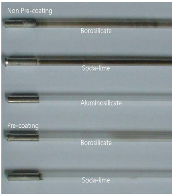
Figure 4. Blackening with Y_2O_3 pre-coating and without coating.
