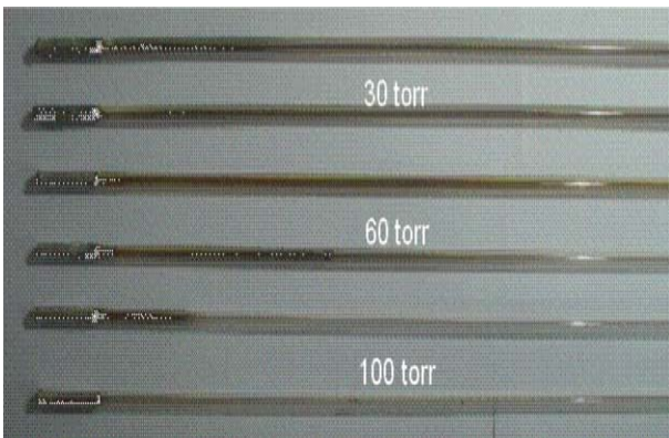
Figure 3(a). Blackening with borosilicate glass tubes of gas pressure 30, 60, and 100 Torr.
