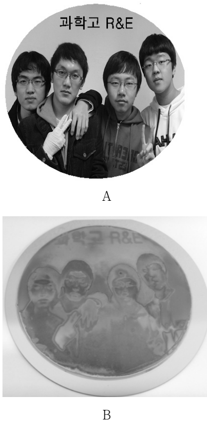
Fig. 7. A; Patterned mask used real photograph, B; porous silicon encoded with optical images.
