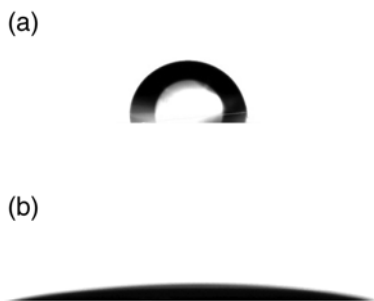
Figure 2. Contact angles on the surface (a) before and (b) after O 2 plasma etching. (50 mTorr, rf power=100 W)
