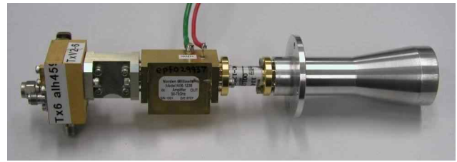
Fig. 3. Photograph of the transmit RF module assembly.
