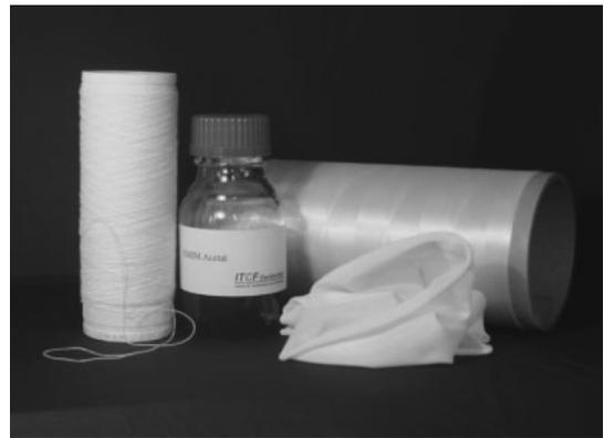
Figure 7. Cellulose fiber obtained by dissolving cellulose in [EMIM]AcO.
