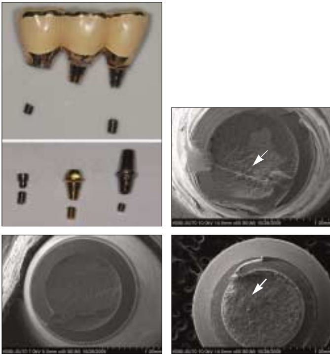
Fig. 1. Clinical images and SEM images of fractured screws. Arrow indicates the starting point of crack line.
