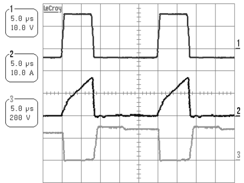
(b) Switch current i_s [2] and voltage v_s [3]
