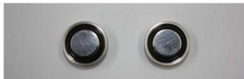
Figure 3. Photo of two sonic nozzles under test ( $\Phi$  0.03 mm,  $\Phi$ 0.2 mm).
