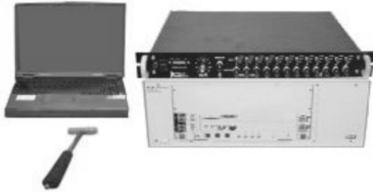
(a) Measuring equipments for natural frequency, acceleration and strain
