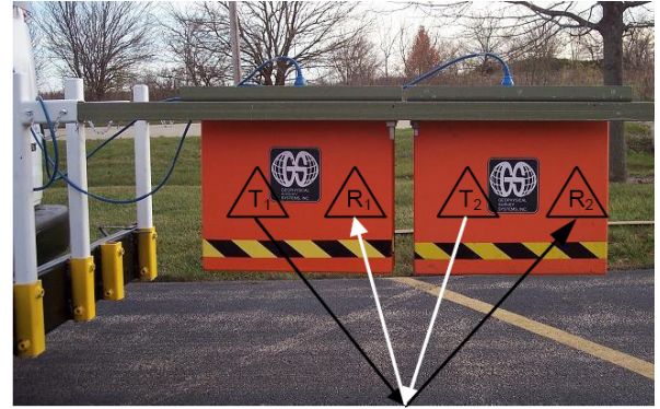
Fig. 3 2.0GHz air-coupled GPR antenna arrangement for the XCMP method (Leng, 2011)
