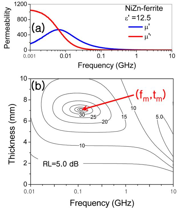
Fig. 2. (Color online) (a) Real ( $\mu'$ ) and imaginary ( $\mu''$ ) permeability spectra of the NiZn ferrite material. (b) Contour map of the return loss with sample thickness and frequency in NiZn ferrite material. The matching frequency ( $f_m$ ) and matching thickness ( $t_m$ ) are indicated at the maximum return loss.
