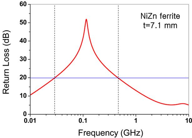
Fig. 3. (Color online) Return loss with frequency for NiZn ferrite material with  $t = 7.1$  mm.
