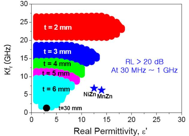
Fig. 4. (Color online) Material parameters of  $Kf_r$  and  $\epsilon'$  satisfying the 20 dB return loss in the frequency range of 30 MHz~1 GHz. The material parameters of NiZn ferrite and MnZn ferrite are indicated for the comparison.
