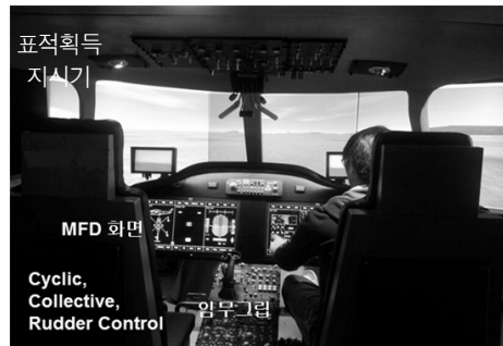
Fig. 1. Simulator Cockpit of Armed Helicopter
