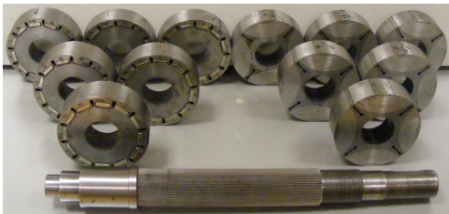
Fig. 4. The photograph of the magnet and reluctance pieces and the rotor shaft
