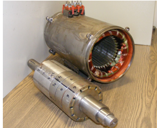
Fig. 5. The photograph of the hybrid motor structure for the rotor Hybrid3 at the \beta value of 0^\circ
