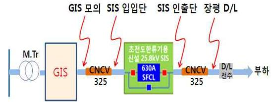
Fig. 2. Schematic of the simulation for Lightning impulses Modeling with SFCL system.
