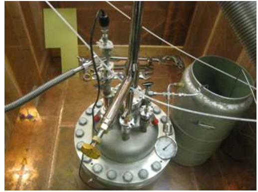
Fig. 2. Photograph of cryostat. The flexible steel hose connects the pressure vessel with the vacuum pump(not shown).
