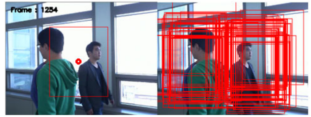
(a) Result of particle filter using color histogram and HOG descriptor.
