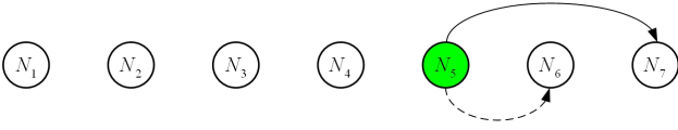
Fig. 4. The relay N_5 transmits the packet to the destination at the third stage.
