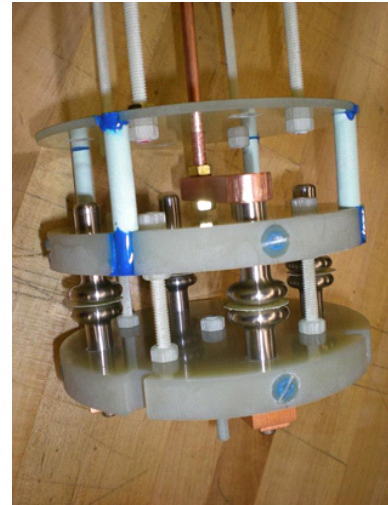
Fig. 2. Carousel type electrode system made of GFRP for breakdown and flashover test.
