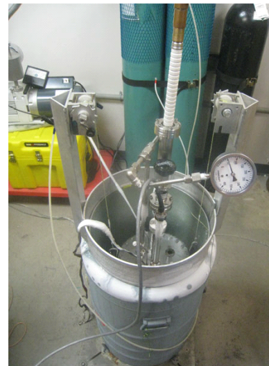
Fig. 3. Pressure vessel in an open cryostat of LN 2 .
