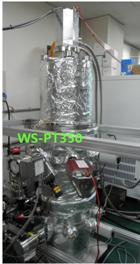
Figure 7. Double dome standard test chamber and prototype cryopump (WS-PT350) installed on it.
