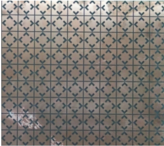
Fig. 3. Part of the fabricated reflector using the designed AMC cell.
