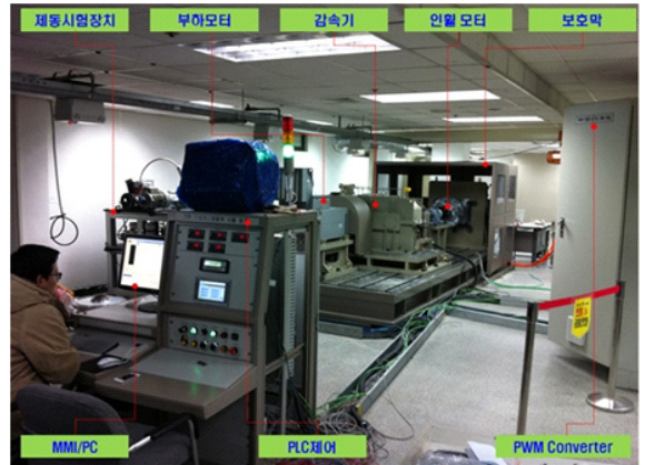
Fig. 8. Control algorithm test using HIL simulator
